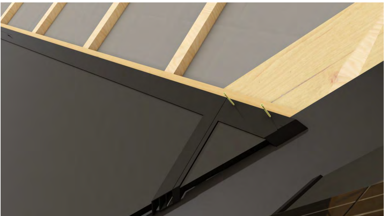
If small triangular infill pieces are required to complete the roof area where mounting clamps cannot be installed, the dummy panel may be fastened directly to the batten. Secure the dummy panel by driving a 5 × 70 mm screw through the upper click profile into the batten.
