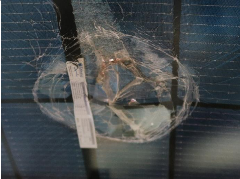
Fig. 7: Solarstone full roof kit, Test set-up (test 1) – Damage back side
