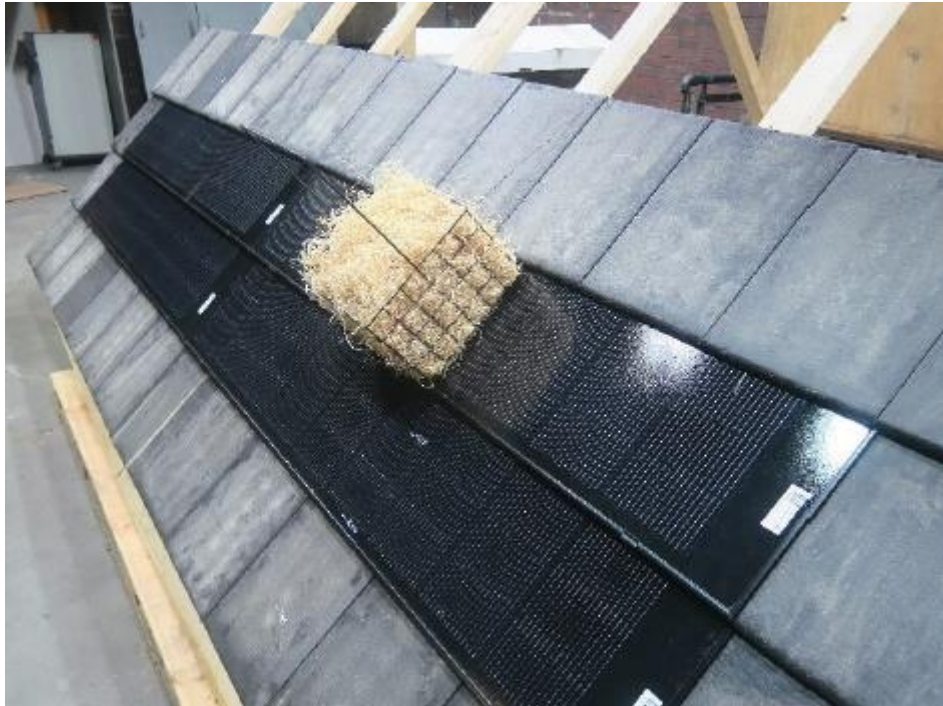
Fig. 17: Solarstone tiled roof kit with PV Modules, Test set-up (test 1)
