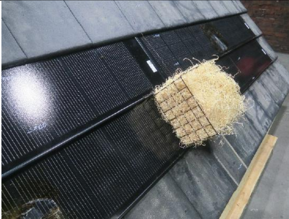
Fig. 25: Solarstone tiled roof kit, Test set-up (test 3)
