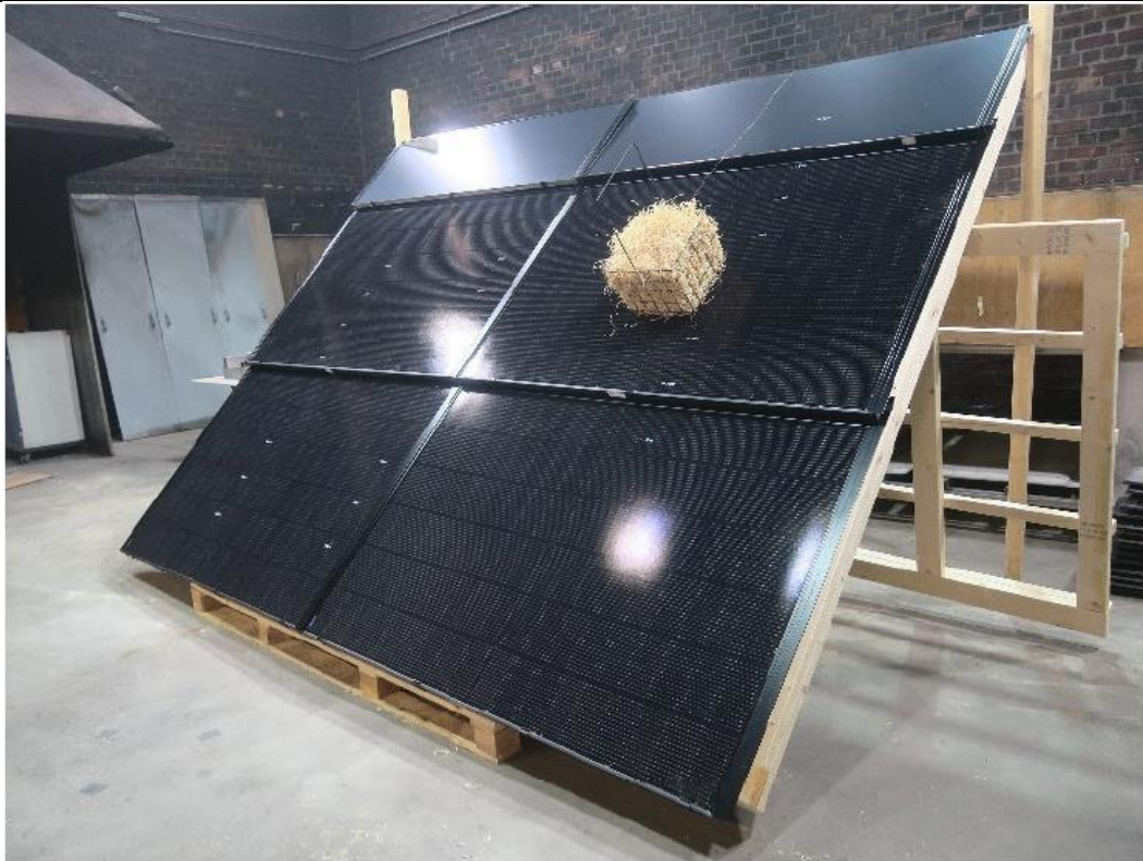
Fig. 3: Solarstone full roof kit, Test set-up (test 1)
