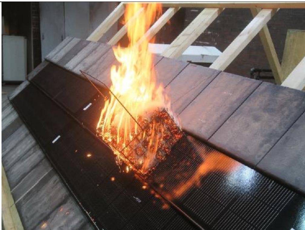
Fig. 18: Solarstone tiled roof kit, Test set-up (test 1) - Ignition
