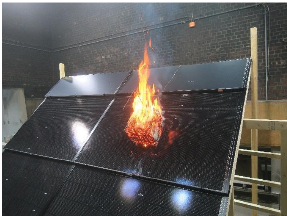
Fig.4: Solarstone full roof kit, Test set-up (test 1) - Ignition
