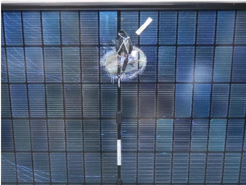
Fig. 12: Solarstone full roof kit, Test set-up (test 2) – Damage back side
