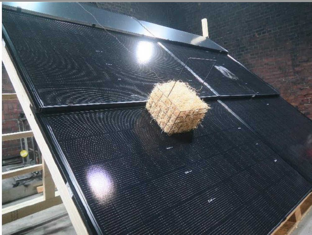
Fig. 8: Solarstone full roof kit, Test set-up (test 2)
