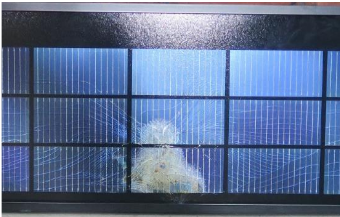
Fig. 24: Solarstone tiled roof kit, Test set-up (test 2) – Damage back side
