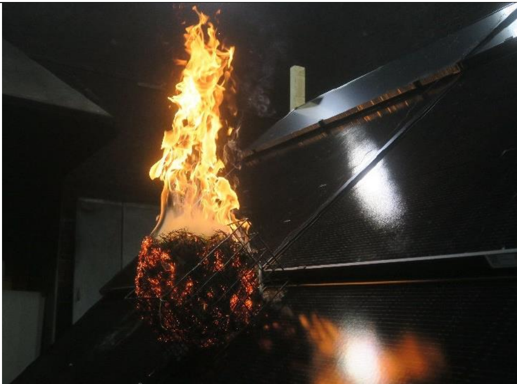
Fig. 14: Solarstone full roof kit, Test set-up (test 3) – Ignition
