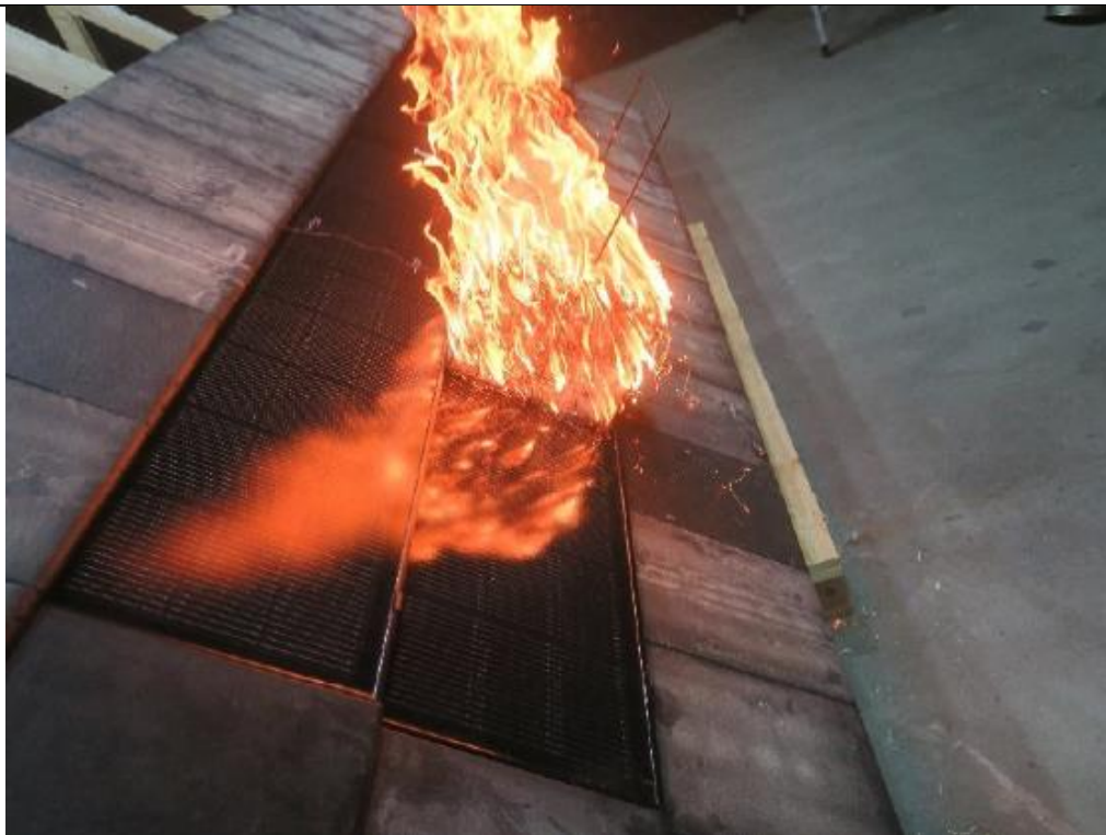
Fig. 22: Solarstone tiled roof kit, Test set-up (test 2) - Ignition
