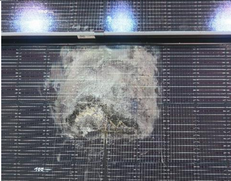
Fig.11: Solarstone full roof kit, Test set-up (test 2) – Damage front side
