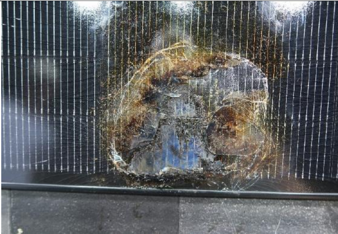
Fig. 23: Solarstone tiled roof kit, Test set-up (test 2) – Damage front side
