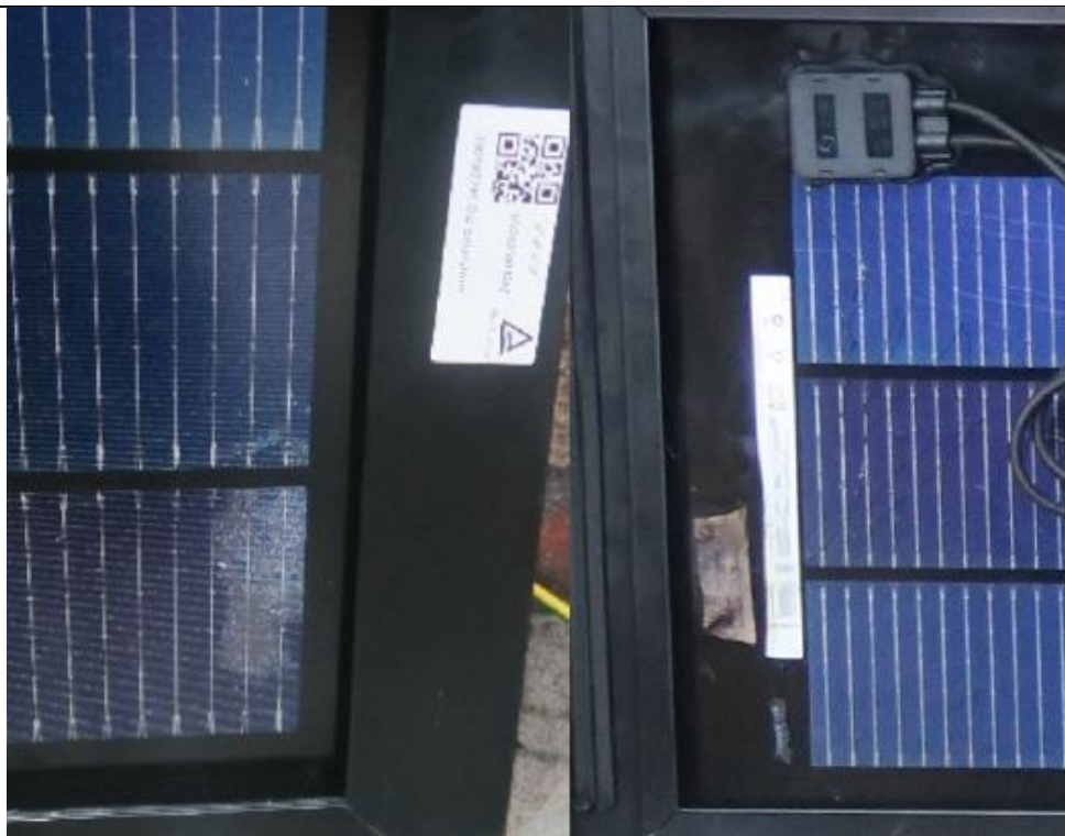
Fig. 28: Solarstone tiled roof kit, Test set-up (test 3) – Damage back side
