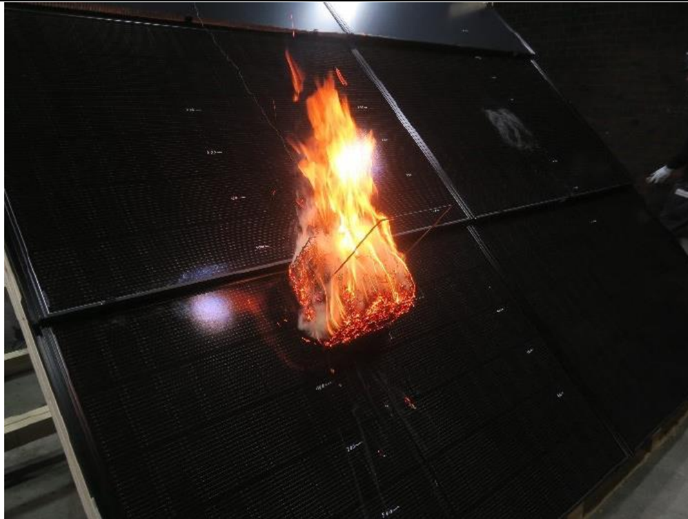
Fig. 9: Solarstone full roof kit, Test set-up (test 2) – Ignition
