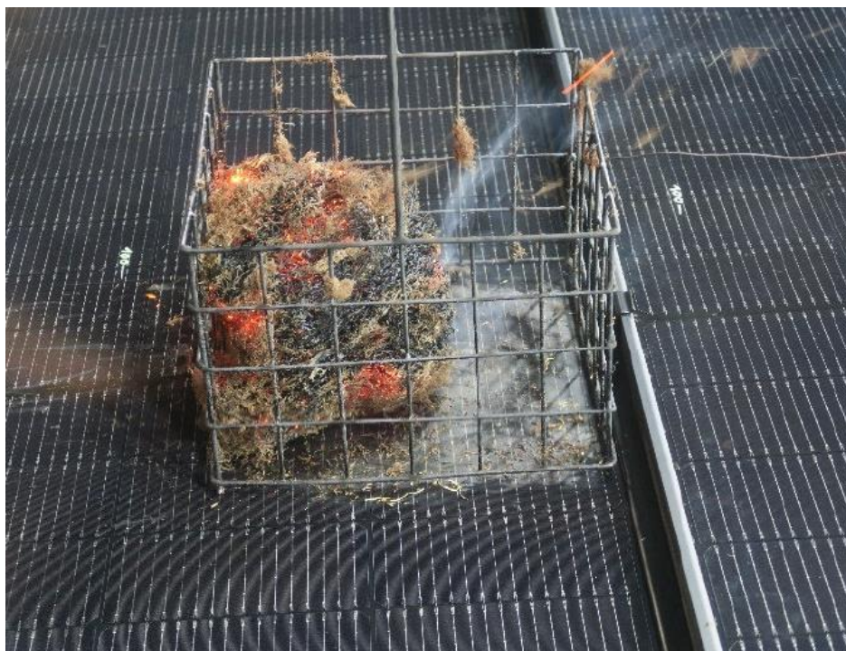
Fig. 10: Solarstone full roof kit, Test set-up (test 2) – During test
